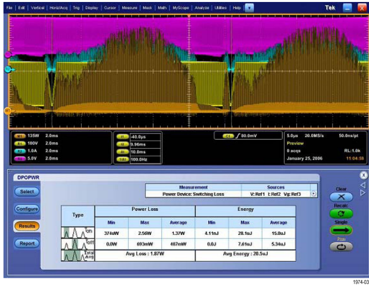
Figure 5: Switching loss results display
